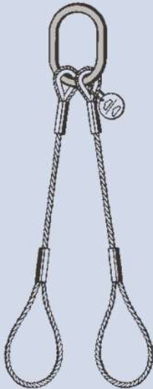
1214. 2-leg wire rope sling with loops
